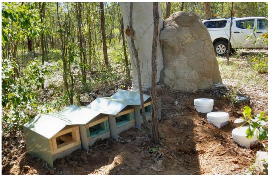
Illustration 1: Test of model houses with timbers treated against termites near Townsville, QLD.
